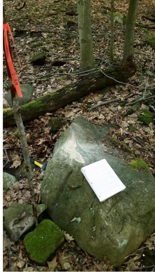
Photo 3.21: Collection of sample from large boulder for terrestrial cosmogenic nuclide (TCN) dating.
