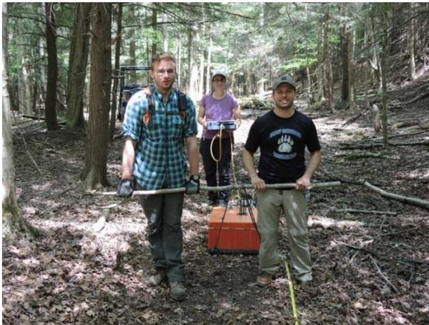
Photo 3.9: Assistants dragging ground penetrating radar (GPR) antenna for 200 MHz data collection.
