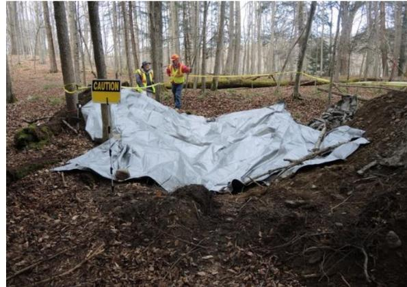
Photo 3.13: Collection of optically stimulated luminescence (OSL) sample in darkened excavation under double tarp cover.
