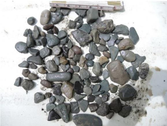
Photo 4.21: Glacial outwash pebble count from pit in glacial depression adjoining the abandoned meander at dated wood site. Note “bright” clast content of limestones, chert, and red sandstone, as contrasted with drab Milkweed Creek clasts seen in other illustrations (such as Photo 3.4).
