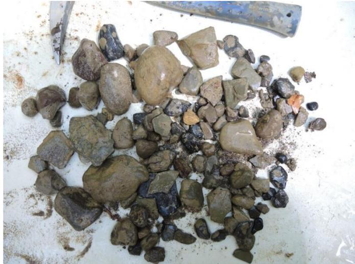
Photo 3.3: Till pebble count from meander depression trench T18; contains “bright” clasts of northerly derivation.
