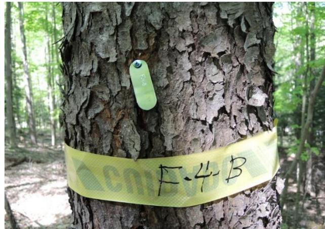
Photo 3.7: Temporary (yellow tape) and permanent (aluminum tags) markers for locations of ground penetrating radar (GPR) survey lines.
