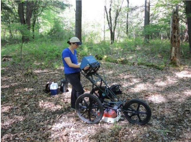
Photo 3.8: Field calibration of ground penetrating radar (GPR) equipment.
