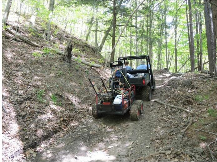
Photo 3.11: UTV vehicle and trailer used to access difficult sites along former logging access roads; some partially regraded during project.
