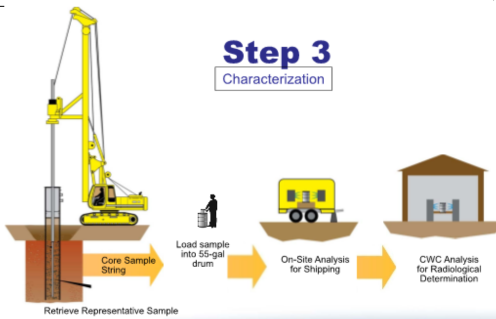
Exhibit V- 8: Sampling and Characterization of Material within a VPU (Dunhan, 2012)
