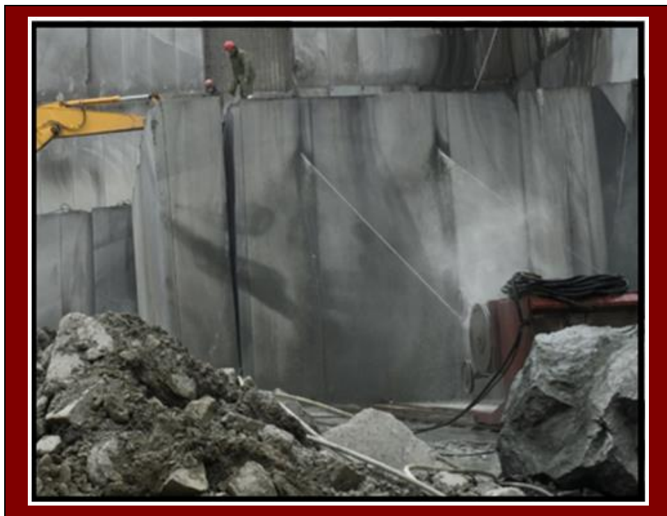
Exhibit VIII-7: Diamond Wire Cutting a Slab in a Quarry
