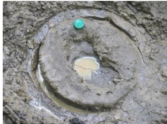
Figure 3. The JET apparatus showing (a) a drawing of the device (Hanson and Cook, 2004), (b) stand-pipe mounted to a tripod, water pump, and local water source (drums), (c) a sealed JET cylinder placed onto a geological material within a dug trench, vertical jet pipe, and point gage, and (d) exposed scour hole (ponded water) once the JET cylinder is removed upon completion of test.
