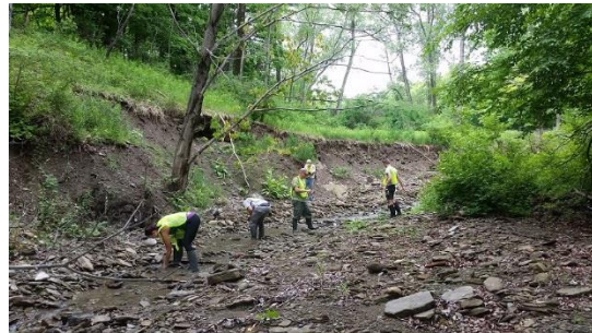
Figure 5. Wolman pebble count method showing (a) pebble axes, where the b-axis is measured, and (b) a typical survey (photo courtesy of T. Zerfas).
