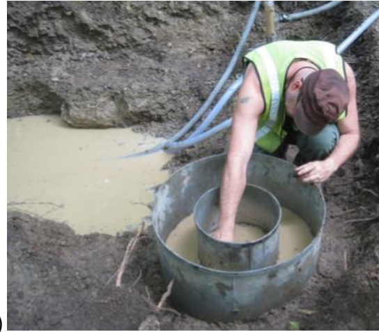
(a) Figure 2. Double ring infiltrometer used in this study showing (a) its components (image from Humboldt), and (b) its application. The manometers were not used.
